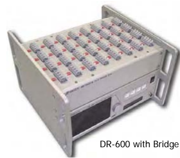
External dimension of amplifier module 24.8W x 95H x 151.5D mm
