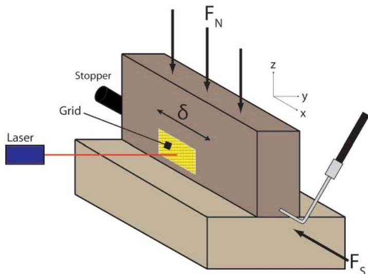
A laser was used to measure local slip,  $\delta$ .
