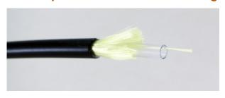
PVC over Kevlar over PolypropylenE. Kevlar fibers prevent stretching. Good for small fiber sensors, D20 & RC20 or smaller. MRI compatible, liquid tight, light crush resistance, but will kink in sharp bends.
