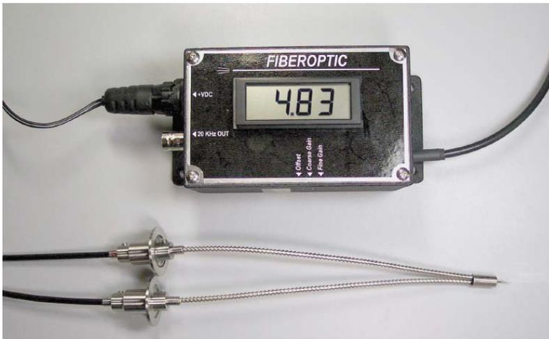
These have the advantage of **small size** (1" diameter) when compared to the Bv2 (2.75") and Bv3 (3.38") passthru designs.
