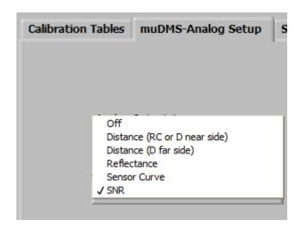
With Option A, muDMS units are provided with two user selectable voltage outputs having a span of 0 to 4.1 volts full scale. These are provided on two BNC connectors. These outputs are factory set to provide the Distance Output and the SNR voltage.
