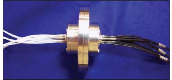
In the BvF vacuum passthru, a Ø 25 mm fused fiberoptic glass rod is used to pass the sensor's light signals thru a vacuum chamber bulkhead. The fused fiber element is a solid glass rod manufactured from fibers that are drawn together with heat and pressure. The rod contains no impurities or voids, is blemish free, and transfers images with zero rotation and distortion, allowing the sensor light signals to be accurately transferred from ambient to vacuum environments.
