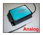
Standard single channel units include amplifier and sensor tip with 914 mm long (3 foot) fiberoptic cable, require +12 VDC input power, and provide 0 to +5 volt analog output with DC - 20 KHz bandwidth.
