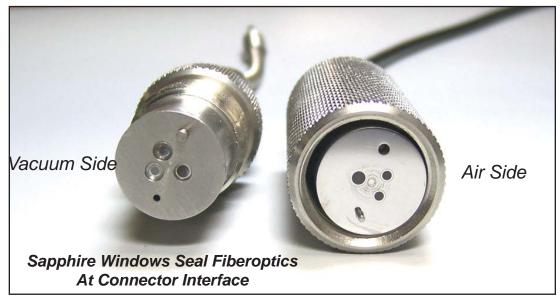
In the Bv1 and Bv133 vacuum passthru, the sensor's transmitting and receiving light guides are separated at a connector interface. This eliminates all crosstalk between channels, thereby allowing the sensor light signals to be accurately transferred from air to vacuum environments. Sapphire windows are epoxied into the connector end on the vacuum side, sealing the fiberoptics in the vacuum.
