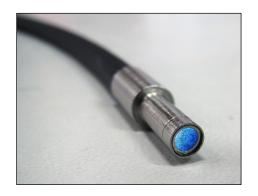
Window probes are used for sensing in high pressure or vacuum applications. Window probes utilize a sapphire window set over the fiber bundle. The window is recessed into the sensor tip and epoxied to the face of the fiberoptic bundle to seal against the high pressure or vacuum.
