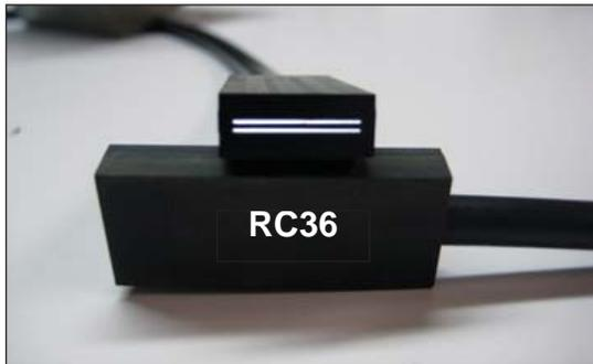
The calibration to a flat surface shows an operating range of about 3 mm.
