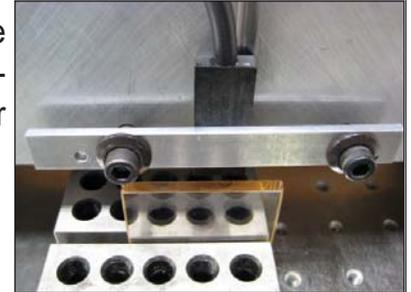
The RC36 tip was mounted above the glass at a gap of 1.2 mm.
