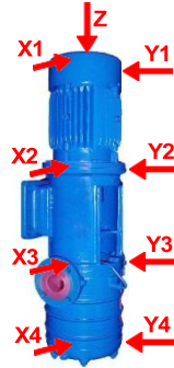
Figure 14: Measuring Points on Machines with Vertical Rotors
