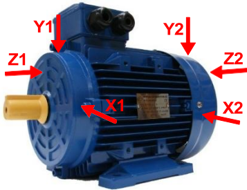
Figure 13: Measuring Points on Electric Motors
