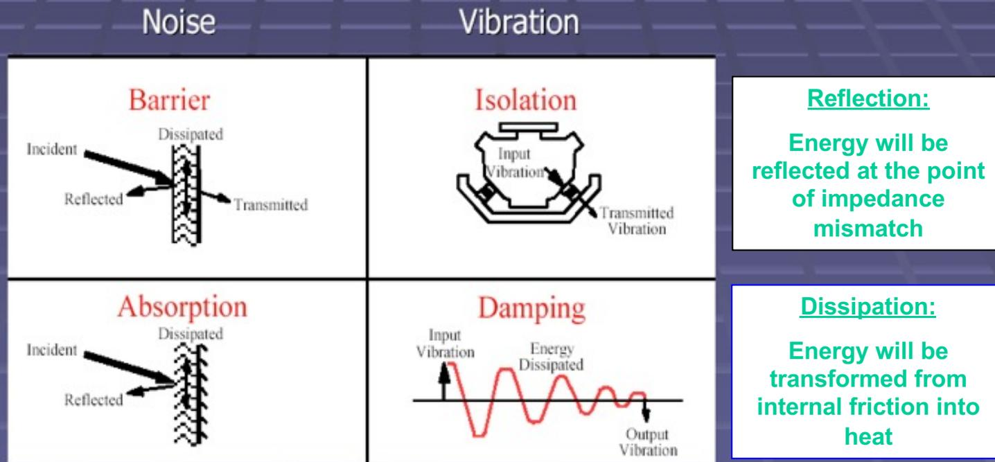
Each material performs a special function to reduce noise or vibration
