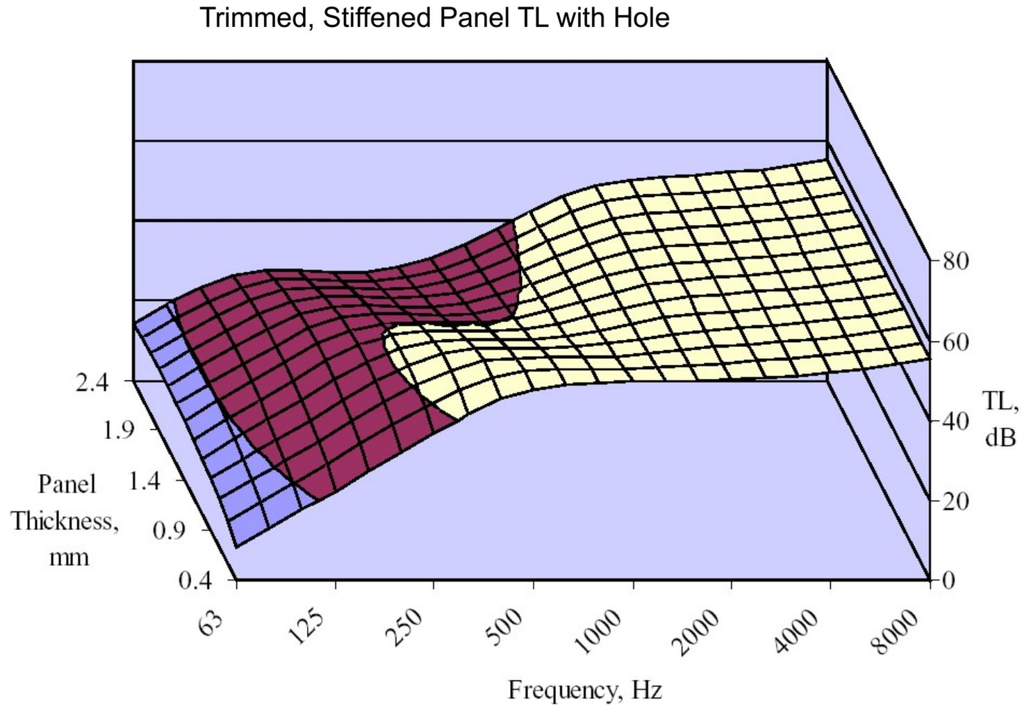
With the stiffened panel the coincidence dip in the TL moves down into the 500Hz range for the larger panel thickness.
