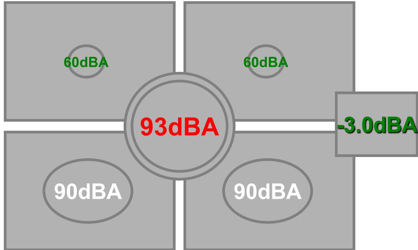
2 sources (or windows) with 90dB sound intensity and two sources with 60dB will sum up to 93dB overall !
