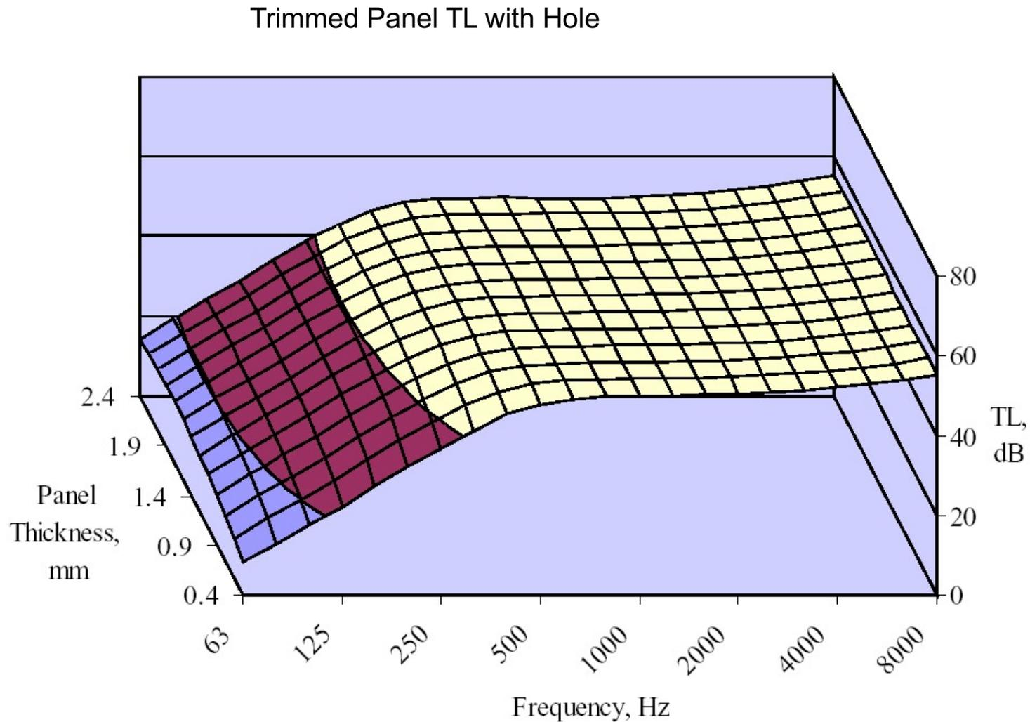
The hole flattens of the TL at high frequencies,
