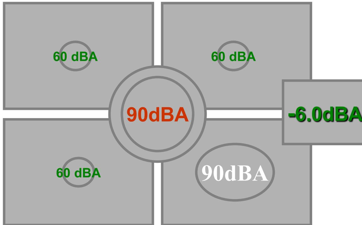
1 source (or windows) with 90dB sound intensity and three sources with 60dB will sum up to 90dB overall !
