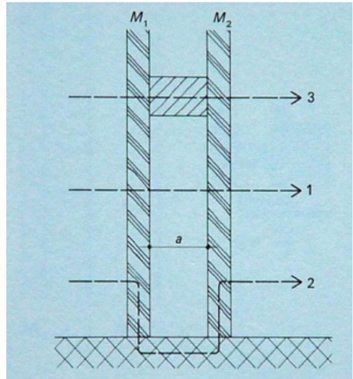
1. Transmission through cavity (air or absorber)
