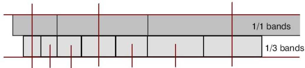
The Lower band limit of a 1/x octave band is  $f_c \cdot 2^{-1/2x}$
