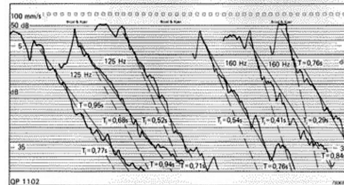
Fig.13. Examples of low frequency decay curves. T is the reverberation time obtained from the slope between -5 and -35 dB levels. T<sub>i</sub> is reverberation time from early decay rate
