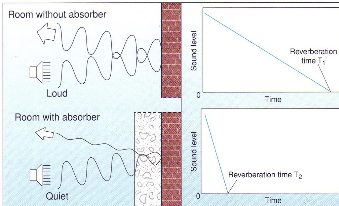
Physically the absorption is achieved due to the conversion of vibrational energy into heat by friction within the material.
