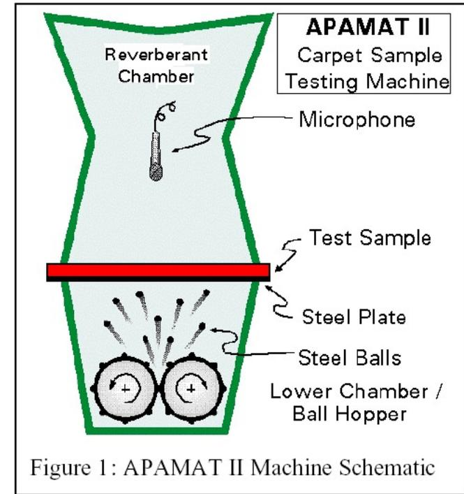
Figure 1: APAMAT II Machine Schematic
