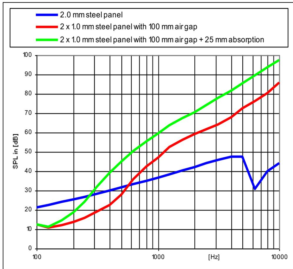
**STL improvement due to absorption in double wall cavity**
