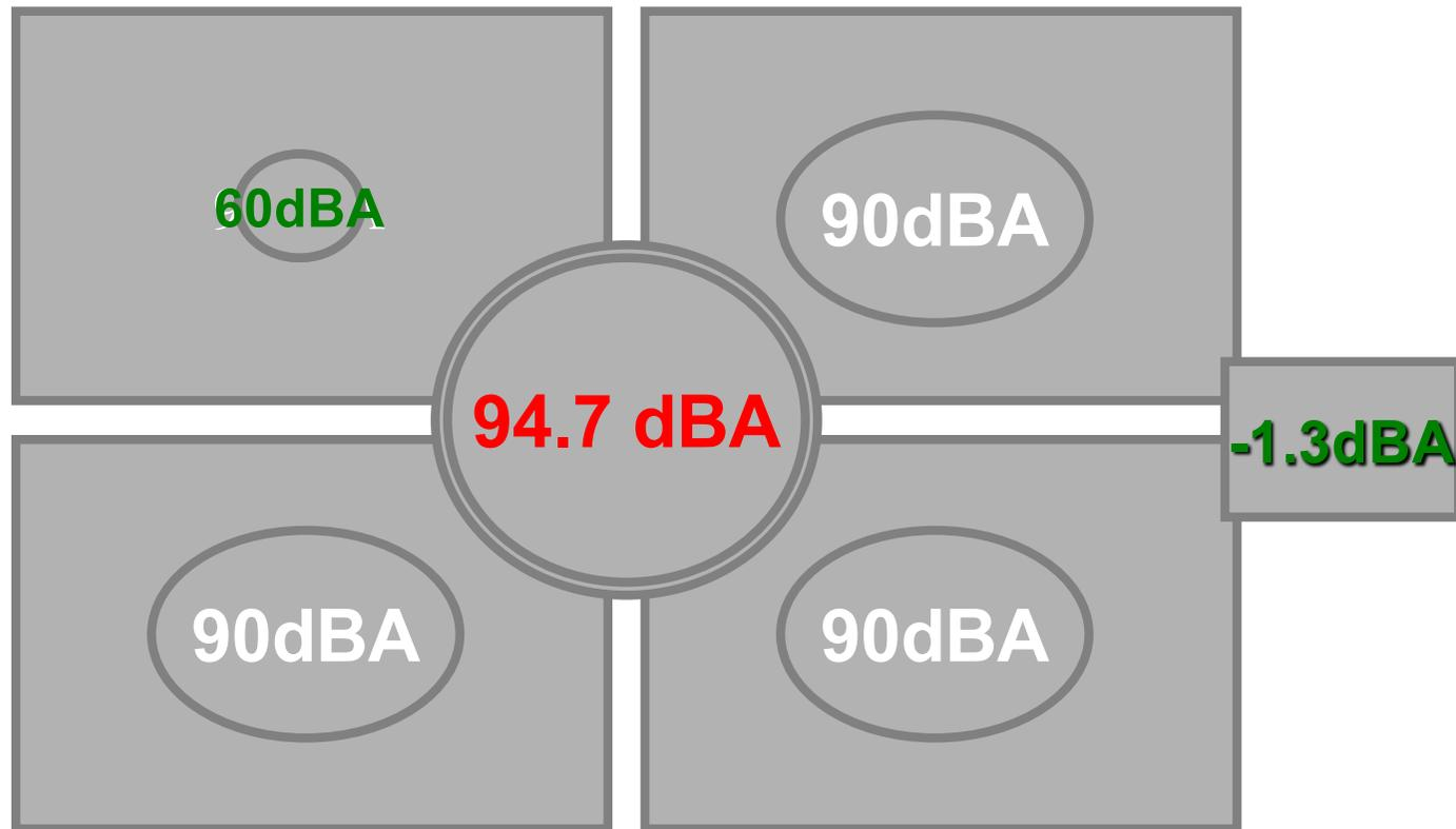
3 sources (or windows) with 90dB sound intensity and one source with 60dB will sum up to 94.7dB overall !
