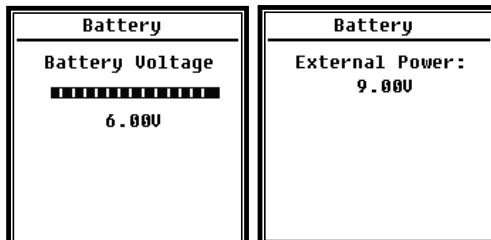
Menu of **Battery** display the power state and power voltage. The discharge cut-off voltage of single cell LR6/AA/AM3 alkaline battery is approx. 0.9V, therefore sound level meter will power off automatically when the total voltage of 4 cell alkaline battery falls below 3.6V.
