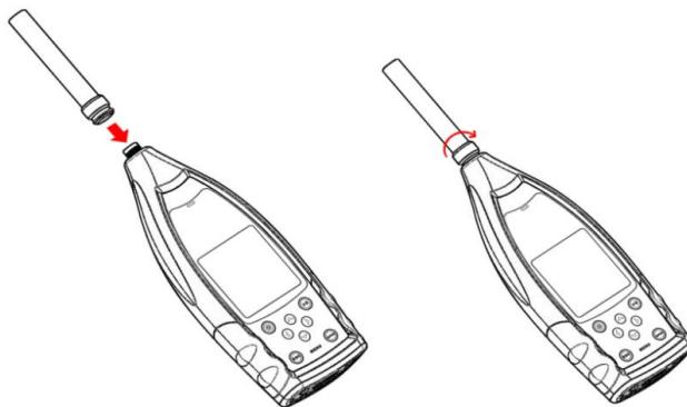
Insert microphone to TNC connector. Then rotate the thread until the connection is tight.
