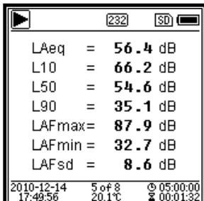
Custom Measurement Page 1. User can set the parameters of the 14 sets of measurement. This screen can display the first 7 sets.
