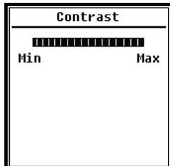
Menu of **Contrast** can set the contrast of LCD display for 14 levels adjustable. Press **<▲>**, **<▼>** can choose and select.
