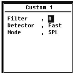
Press **<▲>**, **<▼>** can set the option of each group of custom measurement: **Filter**, **Detector** and **Mode**.
