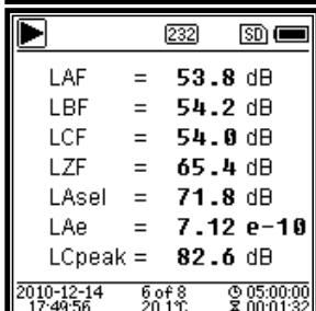
Custom Measurement Page 2. User can set the parameters of the 14 sets of measurement. This screen can display the last 7 sets.
