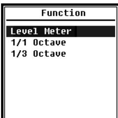
Select **Function** and press <Enter> to enter this menu. 3 kind of measurement can be select: **Level Meter**, **1/1 Octave** and **1/3 Octave**. Press <▲>, <▼> can select mode of measurement. Press <Enter> to save setting and return to previous menu. Press <ESC> to return to previous menu.
