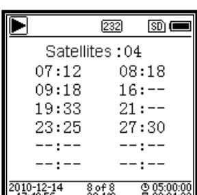
GPS Page 2. Display number of satellite which contribute to positioning, and signal noise ratio of all visible satellites (0dB~99dB).
