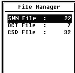
**File Manager** can manage the stored SWN, OCT and CSD file. The numbers display at the right side of each line is the file count for each kind of file type. Press <▲>, <▼> can choose and select, press <Enter> to access next level of menu.
