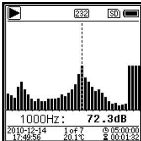
1/3 Octave Spectra. Display 36 bands of 6.3Hz~20kHz and  $L_{Aeq}$ ,  $L_{Beq}$ ,  $L_{Ceq}$ ,  $L_{Zeq}$  as bar graph. Press  $<\blacktriangle>$ ,  $<\blacktriangledown>$  to display the detail value of each band. A threshold can be set for each band. The LED indicator will turn red when the data exceed the threshold.
