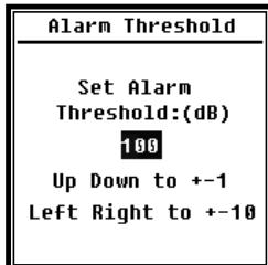
If measurement result of Profile 1~3 exceeds the **Alarm Threshold**, the LED indicator above <Power> will turn red.
