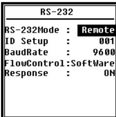
Menu of RS-232 can set the option of serial port, refer to [5. RS-232 Communication Protocol](#) to earn more detail.
