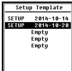
The Setup Template is used to store 5 group user setting parameter of sound level meter for different application.
