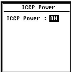
Menu of ICCP power control the 4mA/24V constant current source which can supply all kind of ICCP sensor. Please disable ICCP power before connect to other kind of sensor or directly connect to signal source. Press <**◀▶**>, <**▶▶**> can choose and select.
