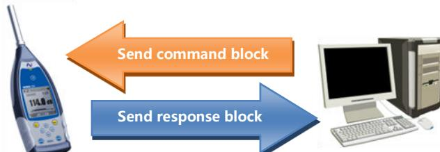
A typical command block or response block consists of “starting character, ID, attribute character, command or data, end character, block check character, carriage returns, line feeds”, as shown below:
