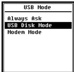
Menu of **USB Mode** can set the working mode when connect sound level meter to computer by USB cable. **Always Ask**, **USB Disk Mode** and **Modem Mode** can be select.
