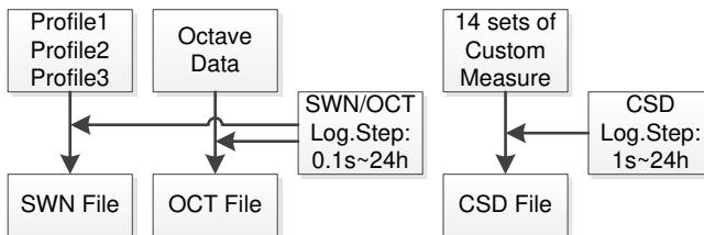
**★Note:** SWN/OCT file only store integral data. The logger step can be considered as the integral period. All the data within logger step (integral period) will be stored as one line into SWN/OCT file. CSD file only store instantaneous data without integration. Once the CSD logger step is reached, 14 group data of custom measure will be stored as one line into CSD file, just as a screenshot.
