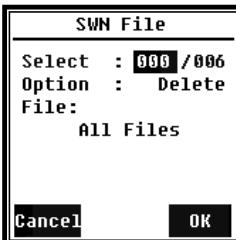
Menu of SWN File can delete SWN files, press <▲>, <▼> to select the file number which want to be delete. The whole file name will be display on the bottom of the screen. Select 0000 as the file
