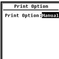
**Print Option** can set the printer option to Auto or Manual. Select **Auto** will print measurement result automatically after stopped measurement.
