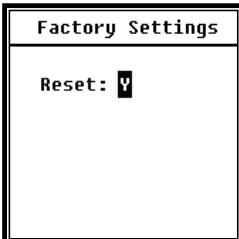
**Factory Settings** provides the function for reset all the parameters which has been modify by users. The parameters will be initialized to the default value. Press <**◀▶**>, <**▶▶**> can select **Y** (Yes) or **N** (No). Choose **Y** and pressing <**Enter**> will initialize the parameter. Choose **N** or press <**ESC**> will cancel the reset.
