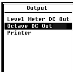
Menu of **Output** can select which measurement data should be output at **DC OUT**. There are **Level Meter DC Out** and **Octave DC Out** option for level meter mode and 1/1 octave mode. The **Printer** option also be include in this menu. Press <**▲**>, <**▼**> can choose and select.
