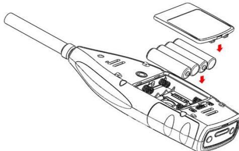
Close and lock the battery compartment after change the battery.
