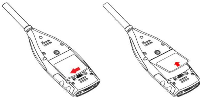
Turn the button to the left side to unlock the battery compartment cover. Then lift the cover to open it.
