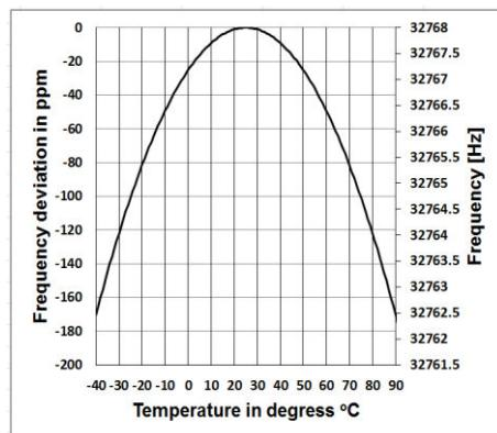
The RTC accuracy may vary by the temperature due to no temperature compensation. As the figure show the typical temperature curve, the RTC keep its basic frequency at 25 °C. When the temperature increase or decrease, RTC frequency change according to  $-0.04\text{ppm}/^{\circ}\text{C}^2$ . Therefore, when the temperature is 0 °C, the change value of RTC is  $-0.04 \times (0-25)^2$
