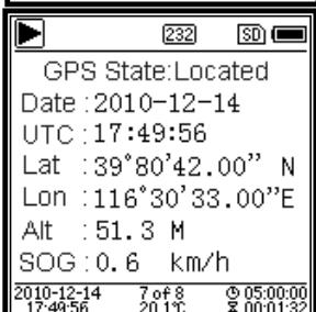
GPS Page 1. Display GPS information: GPS state, GPS date, GPS time, latitude, longitude, altitude and speed.
