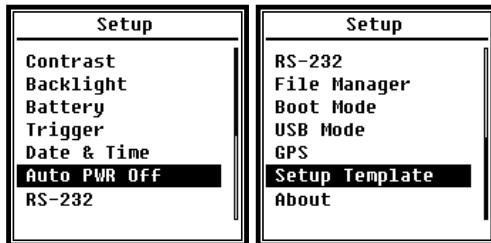
Menu of **Setup** include the basic function setup and condition display. Press **<▲>**, **<▼>** can choose and select, press **<Enter>** to access next level menu.
