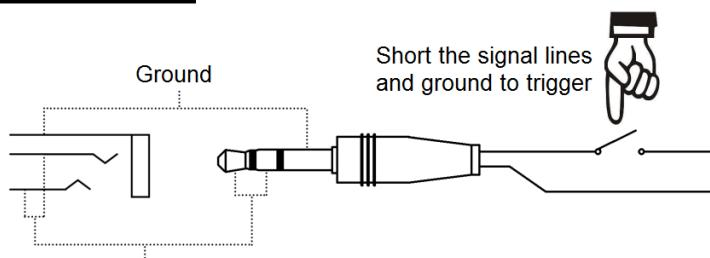
Signal lines, connected together
