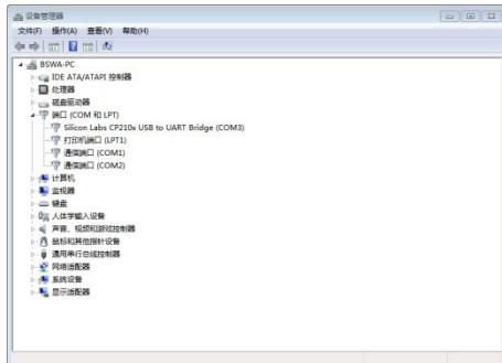
After driver installation, connect sound level meter to computer via USB cable, a new device named **Silicon Labs CP210x USB to UART Bridge (COMx)** could be found in Device Manager.
