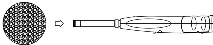
Insert the windscreens onto the microphone until stop according to above diagram. Refer to [Annex 4 Corrections of Windscreens in Free Filed](#) to earn more detail.
