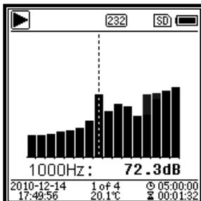
1/1 Octave Spectra. Display 12 bands of 8Hz~16kHz and  $L_{Aeq}$ ,  $L_{Beq}$ ,  $L_{Ceq}$ ,  $L_{Zeq}$  as bar graph. Press  $<\blacktriangle>$ ,  $<\blacktriangledown>$  to display the detail value of each band. A threshold can be set for each band. The LED indicator will turn red when the data exceed the threshold.
