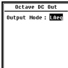
**Octave DC Out** can set the signal output of octave mode. The option is: LAeq, LBeq, LCeq, LZeq and 6.3Hz~20kHz. Press <◀>, <▶> can choose and select. If select unavailable band for current function, it will display "Invalid Octave Band!".
