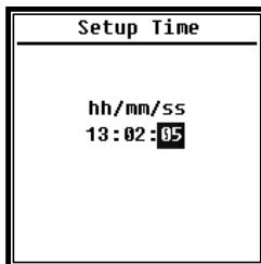
The operation of time setting is almost the same. Press <◀>, <▶> can select hour, minute and second, press <▲>, <▼> can modify the value. Press <Enter> to save the setting.
