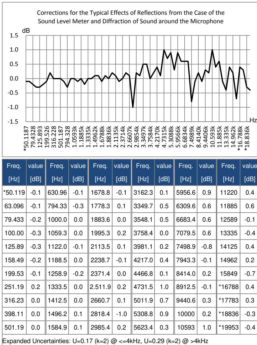
Note: the frequency with \* is not requirement of standard, refer to IEC 61672-1 for exact frequency.
