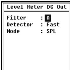
**Level Meter DC Out** can set the signal output of level meter mode. Press <▲>, <▼>, <◀>, <▶> can choose and select.
