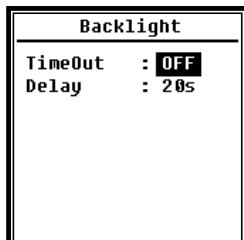
Sound level meter provide the auto turn off function of backlight to reduce the power consume and extend battery life. Menu of **Backlight** can set the backlight timeout on-off and delay time. Press **<▲>**, **<▼>** can choose and select.
