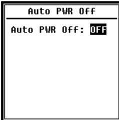
Sound level meter provide the auto power off function to reduce the power consume. When sound level meter keep stop state and no key press for a while, it will power off base on the setting. The Auto PWR Off option: **1min, 5min, 10min, 30min, Off**. Press **<◀>, <▶>** can choose and select, press **<Enter>** to save the setting.
