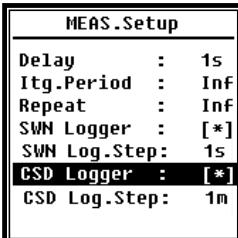
Menu of **MEAS.Setup** is the most important menu related to measurement. It can set the parameter of **Delay**, **Itg.Period**, **Repeat**, **SWN Logger**, **SWN Log.Step**, **CSD Logger** and **CSD Log.Step**. Press <▲>, <▼> can choose and select.
