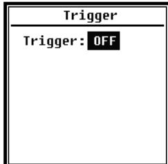
Menu of **Trigger** can set the function of trigger on-off. **Trigger** is an analog input which remote control the sound level meter to start or stop the measurement. The trigger input located on the bottom of sound level meter as a 3.5mm connector.
