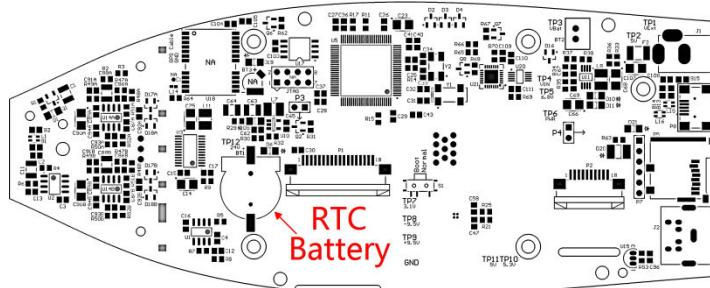
**★Note:** The RTC of sound level meter has calibrated to a reference clock with average error 2ppm (maximum error 3ppm). The time accuracy keep <10ppm (<26s within 30 days) at room temperature. The maximum time error is approx. 5s~8s at 25°C in internal test.
