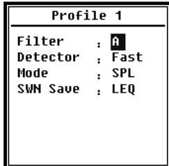
Menu of **Profile 1~3** can set the **Filter**, **Detector**, **Mode** and
