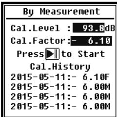
Select **By Measurement** and press <Enter> to enter this menu. Refer to [Annex 2 Adjustments at the Calibration Check Frequency](#) to earn more detail of the stated calibrator and corresponding adjustment value.
