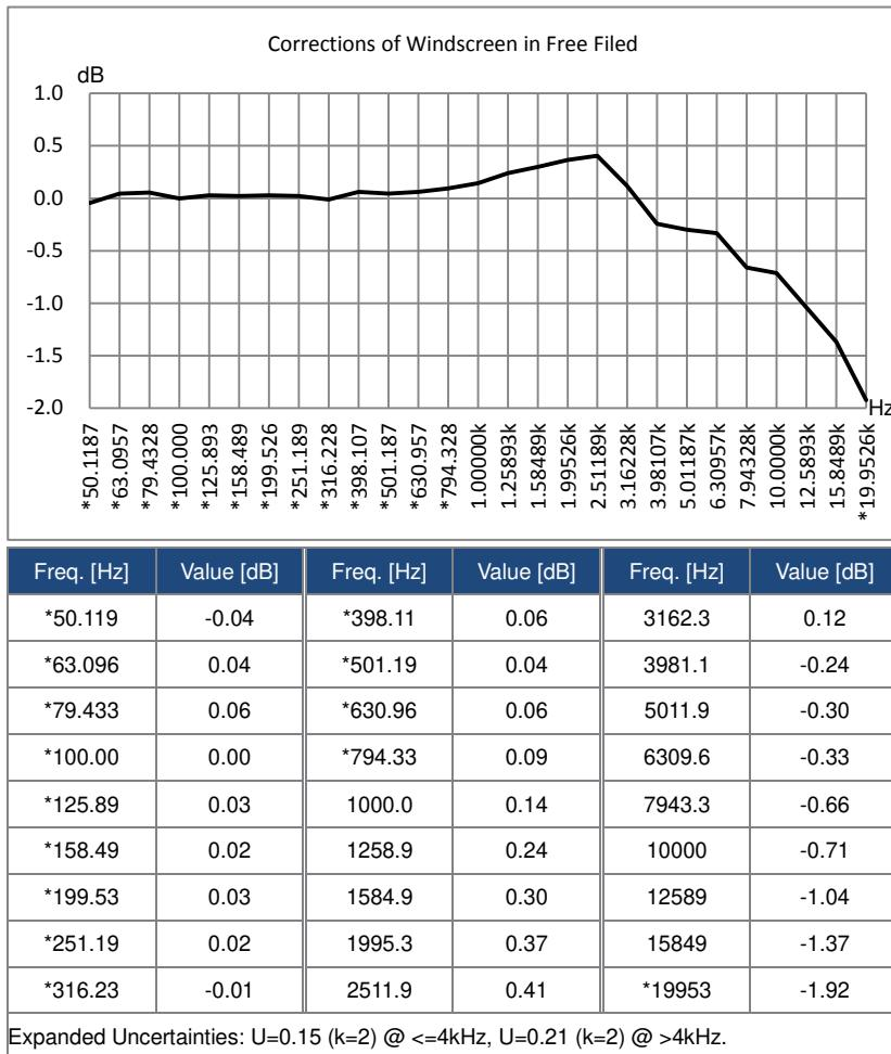
Note: the frequency with \* is not requirement of standard, refer to IEC 61672-1 for exact frequency.
